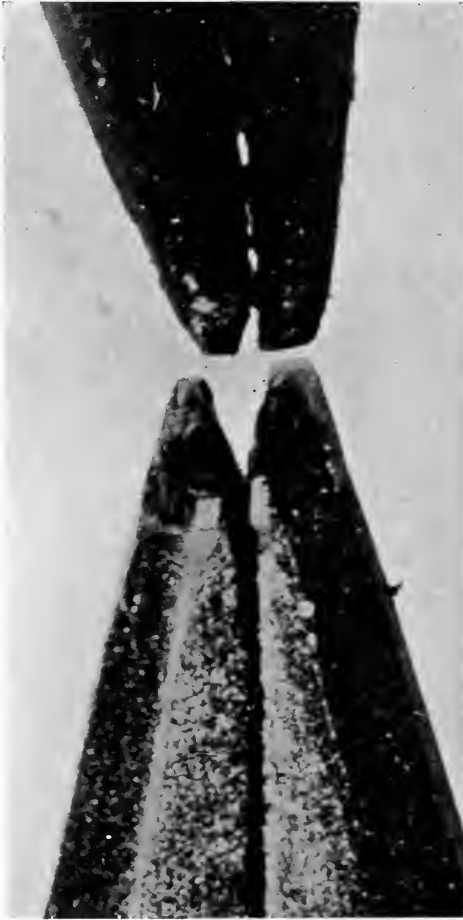
FIG. 78—Comparison of width of pen points. Gold pen with special point and old corroded steel pen. From exhibit in Matter of Frederick C. Hewitt will, Owego, N. Y. Photograph enlarged sixty diameters.
